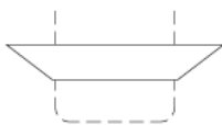
Short Taper Skirt for 2pc. Extended Escutcheon (reduces deflector to ceiling distance by 3/4")
